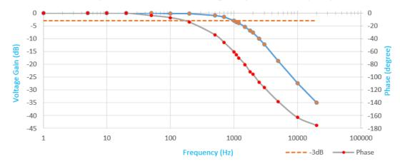
• Find out the cut-off frequency from the plot (where the gain drops to -3dB from its passband value)
