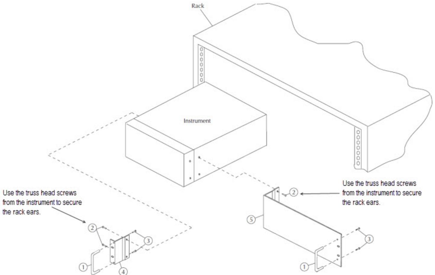
Figure 2: Model 2290-10 suggested single rack fastener installation
