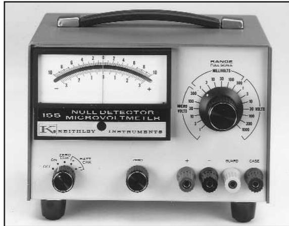
The Model 155 Null Detector/Microvoltmeter is a high-performance, low-cost instrument with better than 150nV resolution and full-scale ranges up to 1kV. Its electrical and physical ruggedness, broad range, and high common- and normal-mode rejection make it one of the most versatile voltmeters available for applications in standards labs, development labs, production testing, and basic research.
