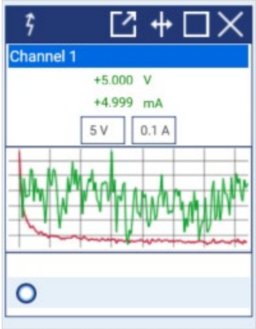
View and set the most essential parameters on the power supply in KickStart's minimized view.
