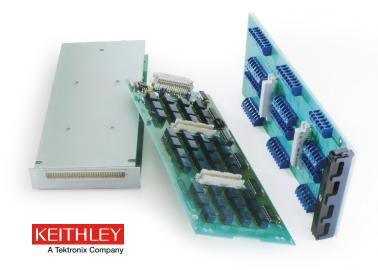
The 7011 40-channel multiplexer has four independent banks of 1×10 switching. Each channel is 2-pole. These four banks can be combined for a wide variety of switching configurations—for example, dual 1×20, or 1×10 and 1×30, or one large 1×40. The 7001 mainframe can automatically configure the 7011 to switch 4-pole signals by combining channel pairs. This gives you a dual 1×10 4-pole multiplexer or a single 1×20 4-pole multiplexer.
