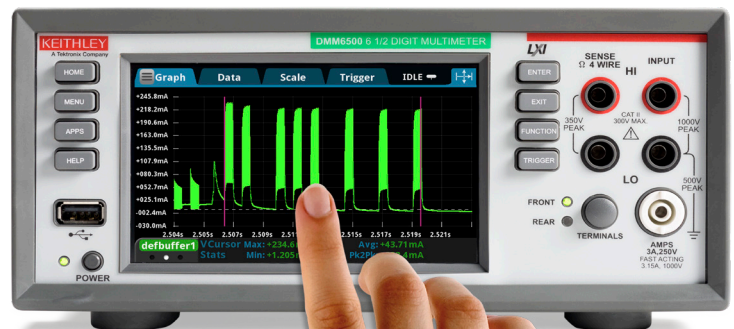
Analyze complex waveforms with the touchscreen display.
