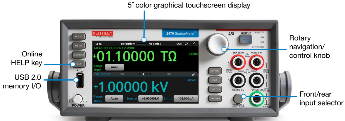
2470 front panel with high-resolution, capacitive touchscreen.
