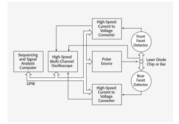
FIGURE 1. This schematic reflects the current testing practices of major laser diode manufacturers. Note that the use of discrete test components increases the integration and programming effort, while severely limiting the flexibility of the test system.
