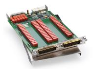
The 3720 offers two independent banks of 1×30 two-pole multiplexers. It is ideal for general purpose switching, including temperature measurements. The two banks can automatically be connected to the Series 3700A mainframe backplane and optional DMM through the analog backplane connection relays. This connection allows the mainframe to reconfigure the card to a single 1×60 two-pole multiplexer or to enable card-to-card expansion for even larger configurations.
