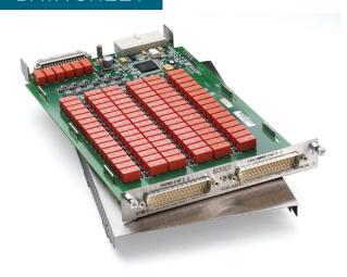
The 3730 is a two-pole, 6 row by 16 column matrix card. It can connect up to six differential instrument channels to any combination of 16 DUTs (devices under test). Any row can be connected to the Series 3700A mainframe backplane by using the analog backplane connection relays. This allows for easy matrix column expansion. A matrix of up to 6 rows by 96 columns can be supported within a single 3706A mainframe (with six 3730 cards).
