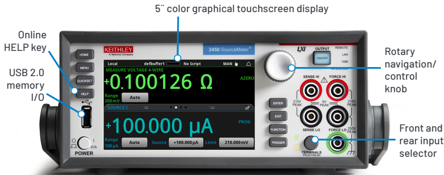
2450 front panel with high-resolution, capacitive touchscreen.
