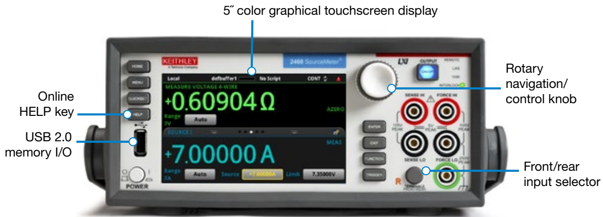
2460-EC front panel with high-resolution, capacitive touchscreen.
