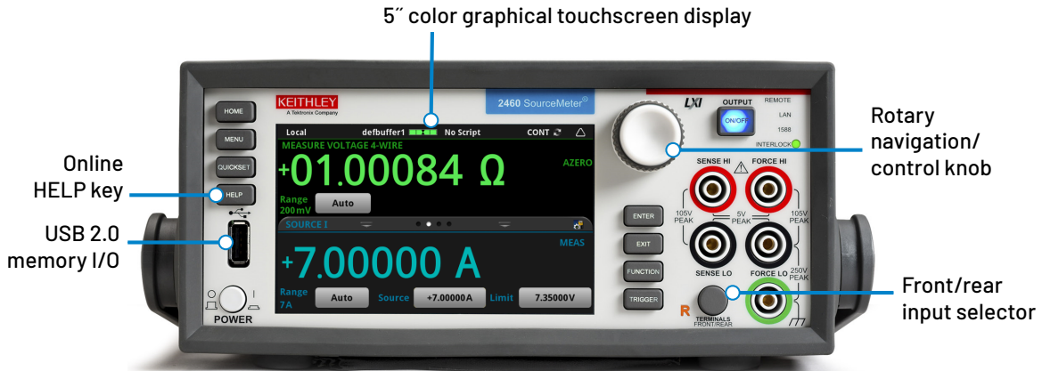
2460 front panel with high-resolution, capacitive touchscreen.
