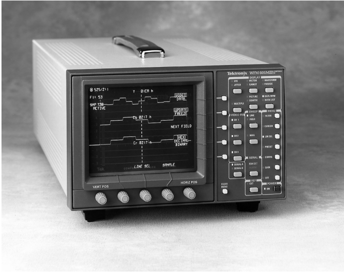
The WFM601M identifies co-sited data values in each channel.
