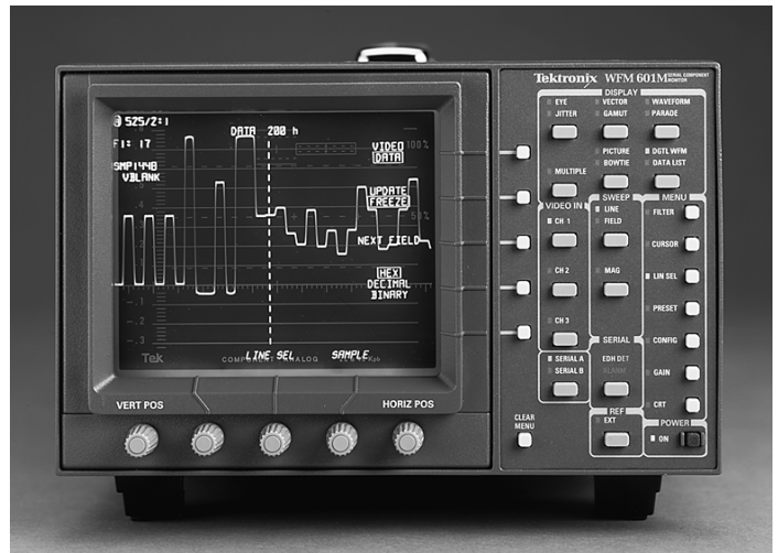
WFM601M wideband data display identifies word values in multiplexed data stream.
