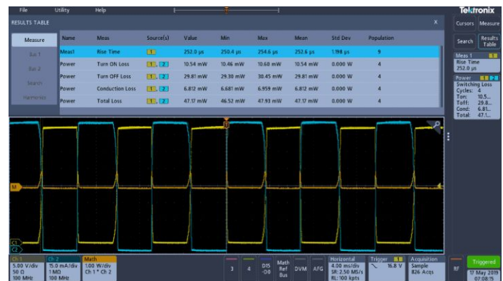
Switching loss measurements
