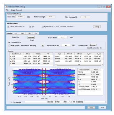
The DSA8300 400G-M4 is a PC based application for PAM4 optical signal validation. The 400G-M4 application supports 4-channel simultaneous acquisition and integrated receiver equalization with support for both autooptimization and user defined equalizer taps values.
