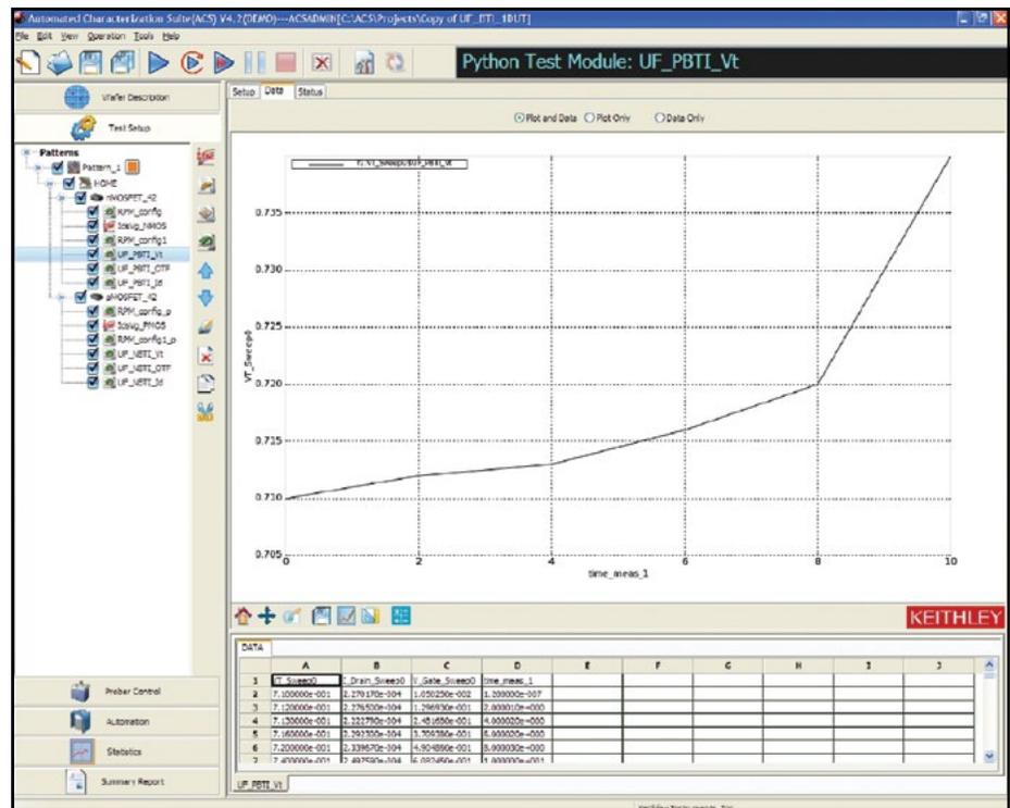
The Model 4225-PMU/4225-RPM's combination of superior speed and sensitivity allow characterizing voltage threshold ( $V_T$ ) directly with high-speed  $I_D$ - $V_C$  sweeps. Measuring  $V_T$  directly makes it unnecessary to correlate the single-point  $I_D$  measurement to actual  $V_T$  levels.
