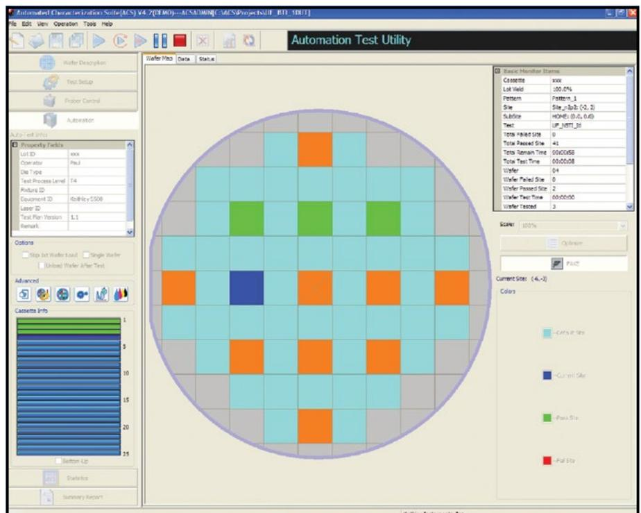
ACS software provides wafer- and cassette-level automation capabilities compatible with semi and fully automatic probe stations.
