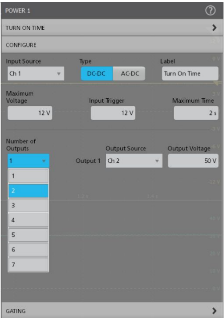
The Turn on time measurement configuration supports multiple output devices
