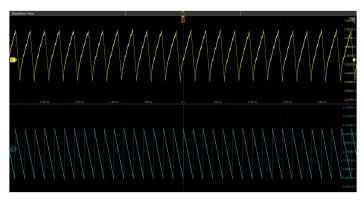
Designers should not confuse Ripple with the System noise. It is possible to see only the ripple by minimizing oscilloscope and probe noise when measuring DC power rails.
