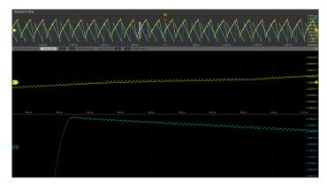
One of the unique features of the DPM solution is the ability to leverage the capabilities of the Power Rail probes to analyze additional high frequency noise overlaid on the ripple. This is typically known as Ripple-on-Ripple.
