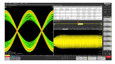
For instance, a SI (Signal Integrity) engineer can measure POL (Point of Load) powering the clock and observe the eye diagram where it is clean and opens up. If the eye diagram is not clean and if there are spurs from POL, then the PI (Power Integrity) engineer can work to modify their power supply design to get better sensitivity. This makes SI engineer see the improvement on the HSS load.
