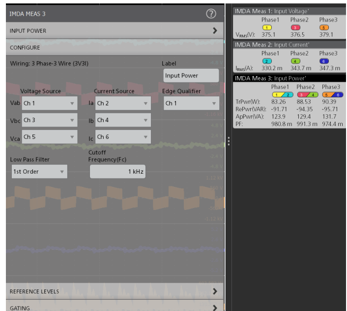
Input analysis wiring configuration
