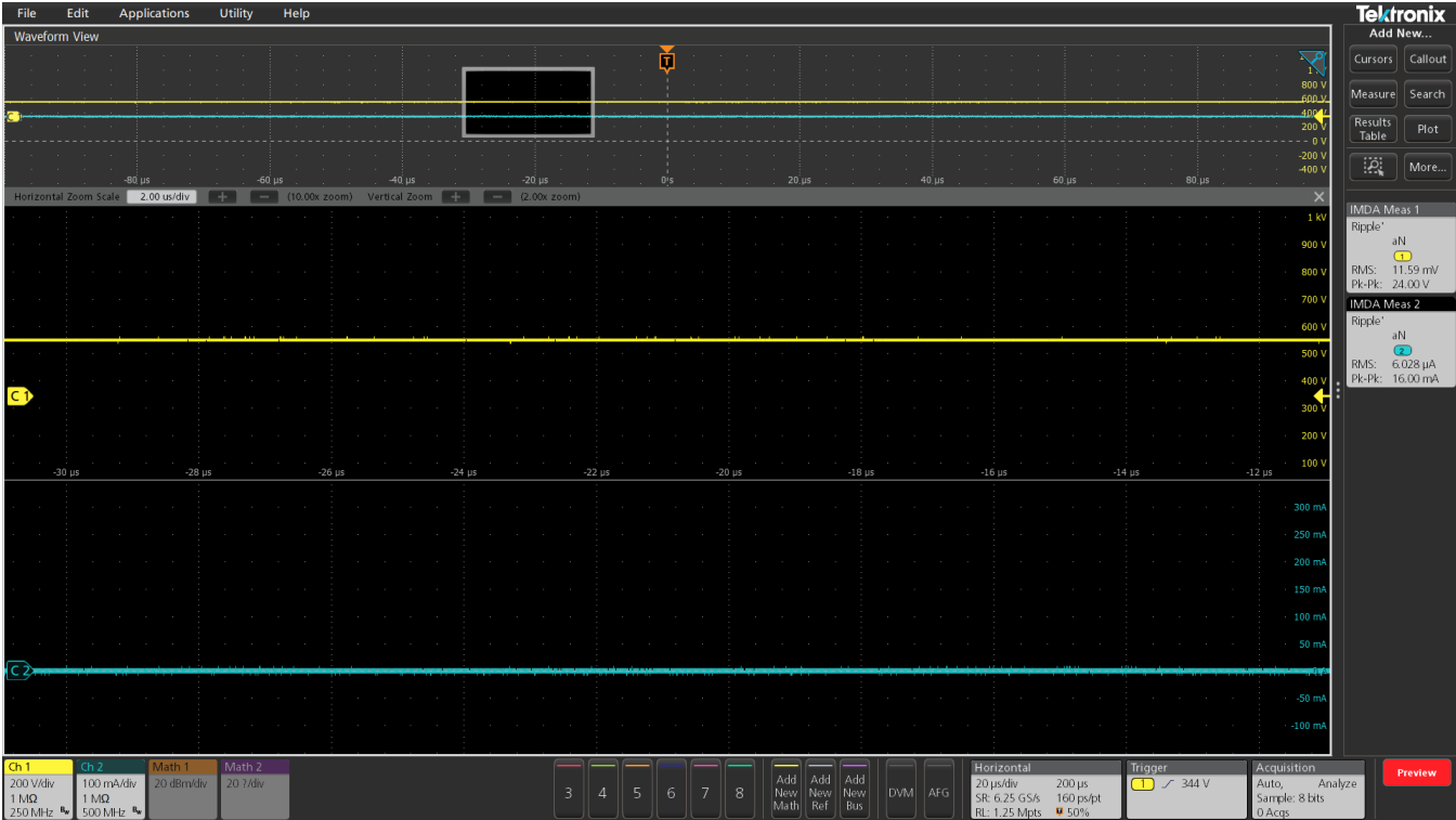
Figure 12: Ripple measurement being carried out on the DC-input signals when testing an Inverter
