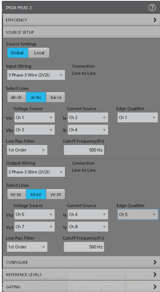
Figure 8: Configure wiring and filters to perform efficiency measurements for an Industrial motor
