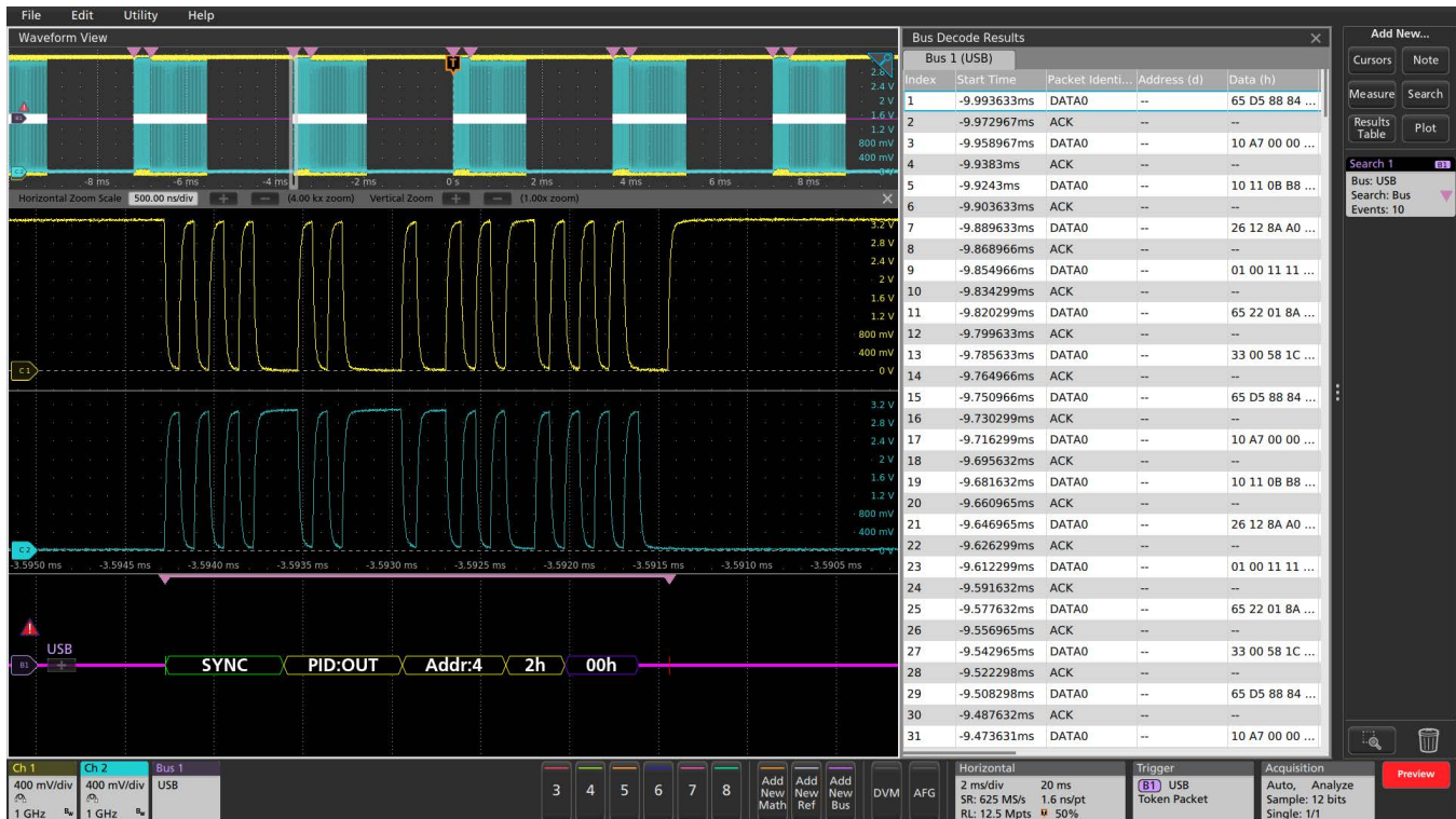
Triggering on a USB full-speed serial bus. A bus waveform provides time-correlated decoded packet content including Start, Sync, PID, Address, End Point, CRC, Data values, and Stop, while the bus decode table presents all packet content from the entire acquisition.
