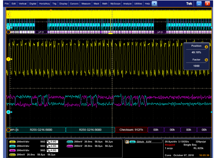
MSO70000C analog-channel decoded display of a Packed Pixel Stream, showing a checksum error.
