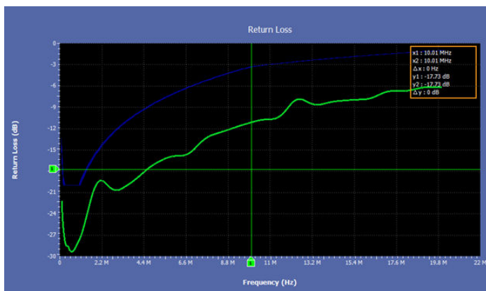
Figure 10: Return Loss plot using Oscilloscope and AWG method
