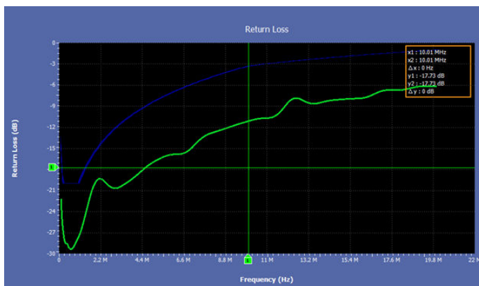
Return loss plot generated using oscilloscope and AWG method
