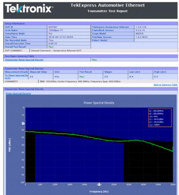
Detailed test report showing PSD mask test plot
