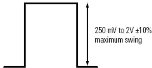
Amplitude swings between 0.25 and 2.0 V allowed; should fit inside shaded area of the following graph. For example, SCFL uses a 0 V termination, and operates between approximately 0 and -0.9 V; as shown with dotted arrow, it falls within the operating range.
