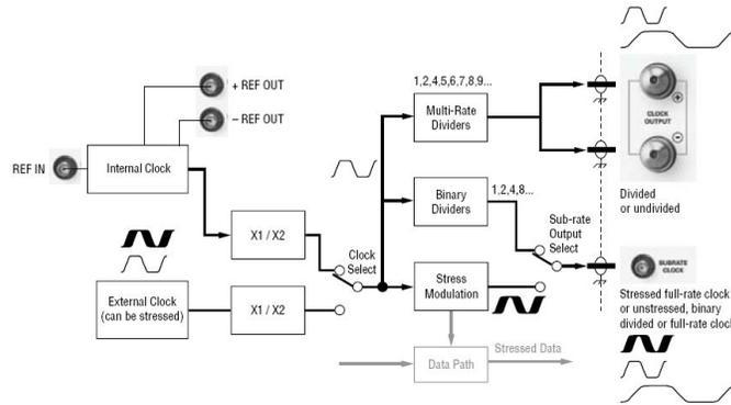
Functional block diagram of the clock path for models with stress capability: BSA125C, BSA175C, BSA286CL.
