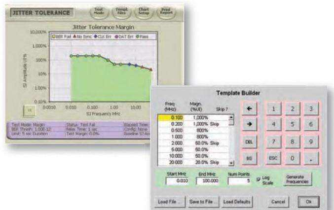
Built-in jitter tolerance function
