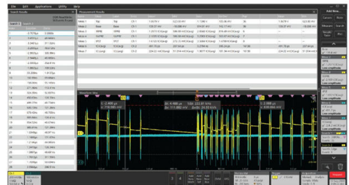
Detailed results showing qualified bursts of a DDR3 signal
