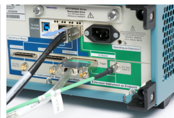
UltraSync connection on instrument with Extension role
