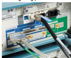
UltraSync connection on instrument with Master role
