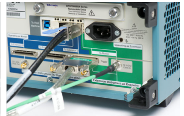
UltraSync connection on instrument with Extension role
