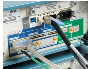
UltraSync connection on instrument with Master role
