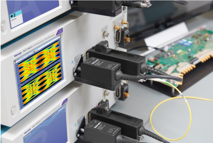
Optical Reference Receiver on a DPO70000SX oscilloscope's ATI Channel
