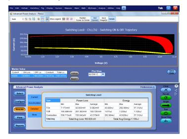
The Trajectory plot for switching loss measurements shows the trajectory of turn-on loss and turn-off loss for all switching cycles.
