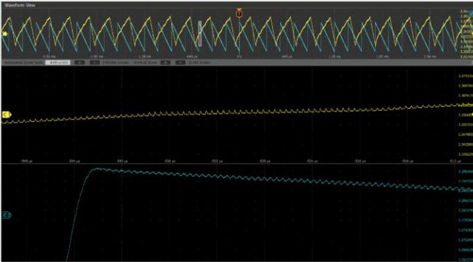
One of the unique features of the DPM solution is the ability to analyze additional high frequency noise overlaid on the ripple. This is typically known as Ripple-on-Ripple.
