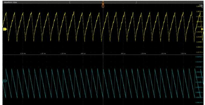
Designers should not confuse Ripple with System noise. It is possible to see only the ripple by minimizing oscilloscope and probe noise when measuring DC power rails.
