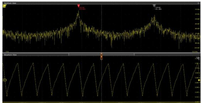
You can analyze cycle-by-cycle by selecting a PWM clock (if available) and view peak-peak and RMS values for each ripple cycle. This gives statistics for all of the cycles within an acquisition. Bandwidth limit capability enables designers to analyze the ripple numbers at different bandwidths.
