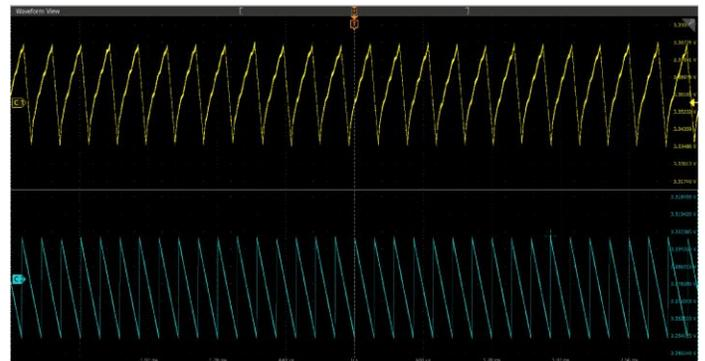
You can perform this measurement for a single cycle within an acquisition or over every cycle within an acquisition (Cycle Mode). You can synchronize cycles based on a power rail signal or another signal in the system. Cycle-by-cycle measurements can be analyzed using statistics, histograms, or plots. Bandwidth limit capability enables designers to analyze the ripple numbers at different bandwidths.
