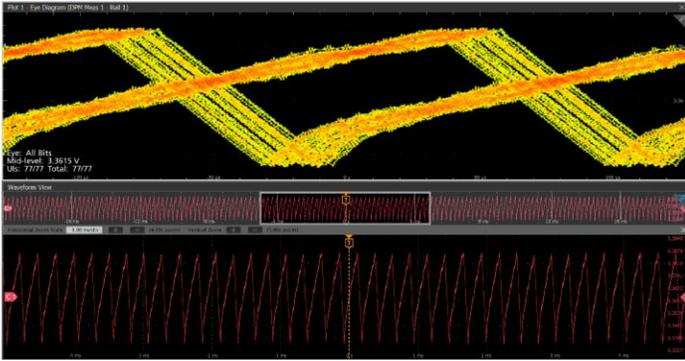
For instance, a signal integrity engineer can measure POL powering the clock and observe eye diagram where its clean and opens up. If eye diagram is not clean and if there are spurs from POL, then the PI engineer can work to modify their power supply design to get better sensitivity. This makes SI engineer to see the improvement on the HSS load.
