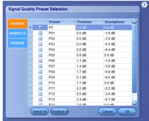
Preset selection panel for signal quality measurements
