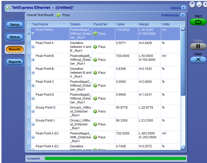
Figure 2: TekExpress Ethernet results panel displaying tests results
