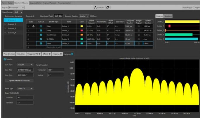
The Tektronix Environment signals plug-in is a simple and flexible tool to create real world scenarios for commercial, electronic warfare, and simulations for monitoring and receiver testing. The plug-in integrates into the SourceXpress waveform creation platform, and the AWG70000 series and AWG5200 series arbitrary waveform generators.
