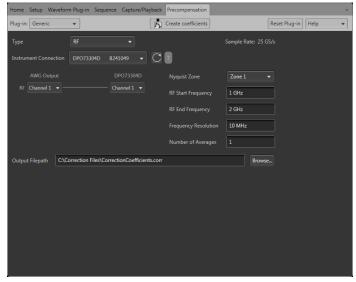
The Tektronix Generic Precompensation application plug-in enhances the capabilities of either the AWG70000A Series Arbitrary Waveform Generators or the SourceXpress<sup>®</sup> waveform generation software, adding the ability to create correction coefficients that can be applied on waveforms to get flat frequency and linear phase response.
