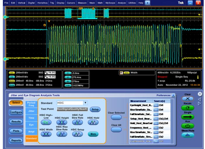
DPOJET automated Opt.HSIC provides 100% test coverage for both Device and Host
