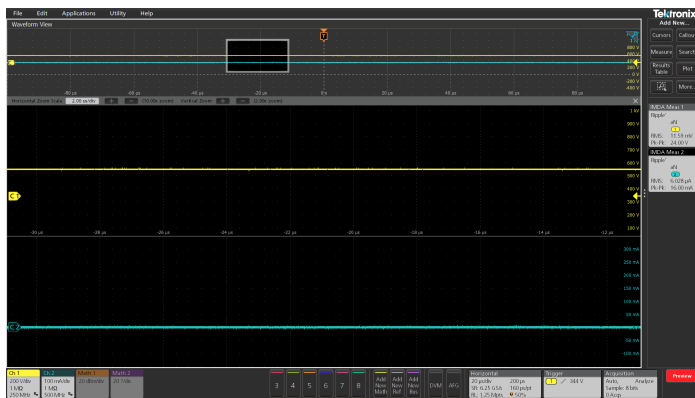
Ripple measurement being carried out on the DC-input signals when testing an Inverter
