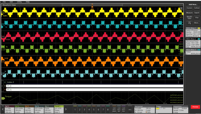
The image shows IMDA application running System Efficiency, Mechanical Power, and Torque measurements using the QEI method
