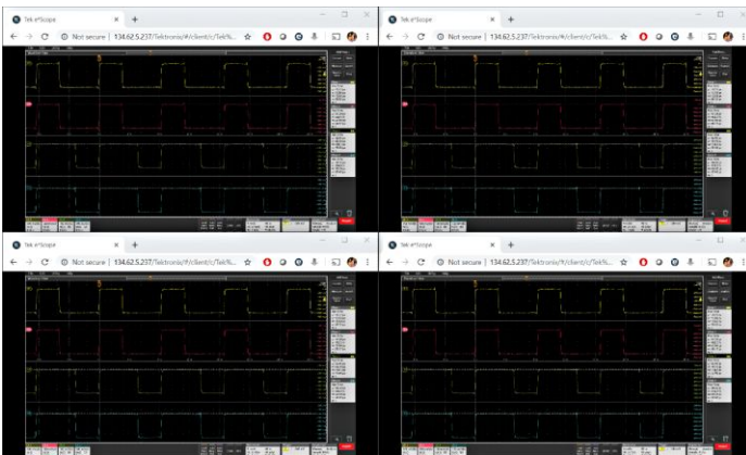
Easy remote control using e*Scope across multiple instruments by tiling browser tabs on a monitor for viewing
