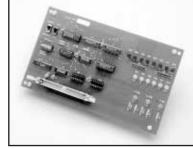
The METRABUS data read-back feature can be tested with the board. Reading data from the MDG-1 will return the last data written to the board without changing it.
