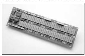
addressable MCPT-8X8 boards from a single METRABUS interface board. Additionally, any number of boards can be assigned the same board address, providing 2, 3 or N pole switches. Relay matrices can, therefore, be expanded in a linear (1 dimension), cartesian (2 dimensions) or geometric (3 dimensions) fashion creating versatile, multidimensional input and control schemes.
