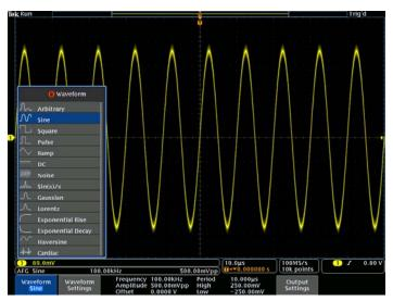
Waveform type selection in the integrated AFG.
