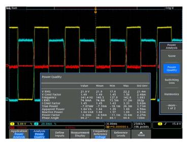
Power quality measurement. Automated power measurements enable quick and accurate analysis of common power parameters.
