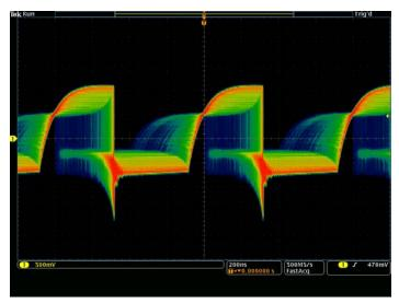
Digital phosphor technology enables a greater than 340,000 wfm/s waveform capture rate and real-time intensity grading.
