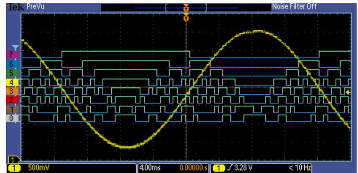
Figure 9: The MSO Series provides 16 integrated digital channels enabling you to view and analyze time-correlated analog and digital signals.
