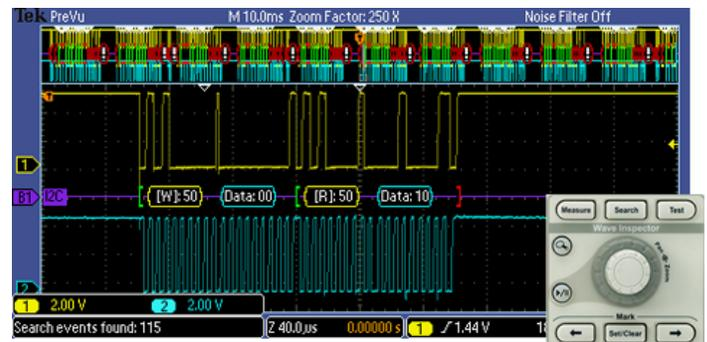
Figure 3: Search - I<sup>2</sup>C decode showing results from a Wave Inspector search for Address value 50. Wave Inspector controls provide unprecedented efficiency in viewing and navigating waveform data.
