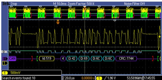
Figure 7: Search step 2: Wave Inspector automatically searches through the record and marks each event with a hollow white triangle. You can then use the **Previous** and **Next** buttons to jump from one event to the next.
