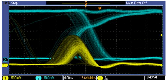
Figure 8: Digital phosphor technology enables a 5,000 wfm/s waveform capture rate and real-time intensity grading on the MSO/DPO2000B Series.
