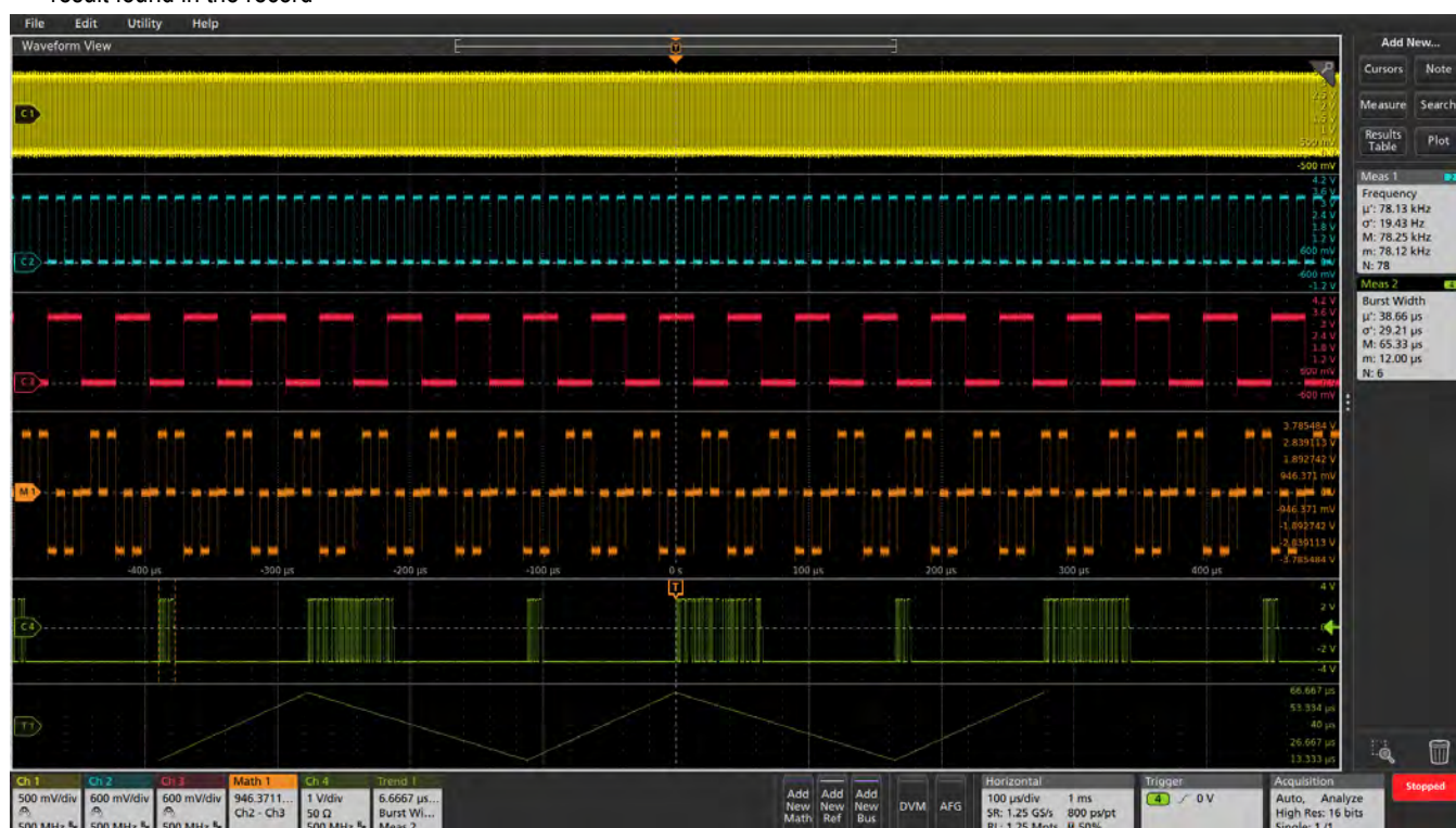
Figure 20: Using measurements to characterize burst width and Frequency.
