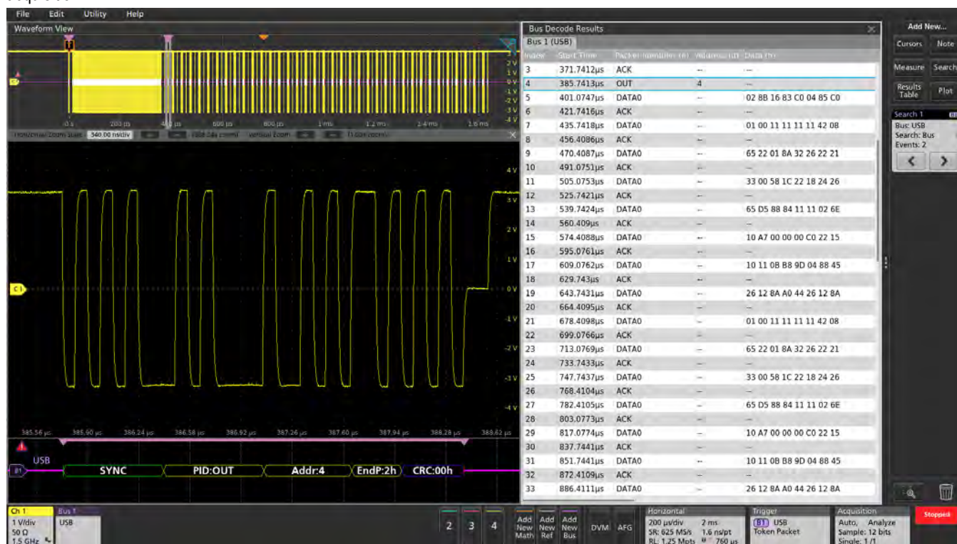
Figure 24: Triggering on a USB full-speed serial bus. A bus waveform provides time-correlated decoded packet content including Start, Sync, PID, Address, End Point, CRC, Data values, and Stop, while the bus decode table presents all packet content from the entire acquisition.
