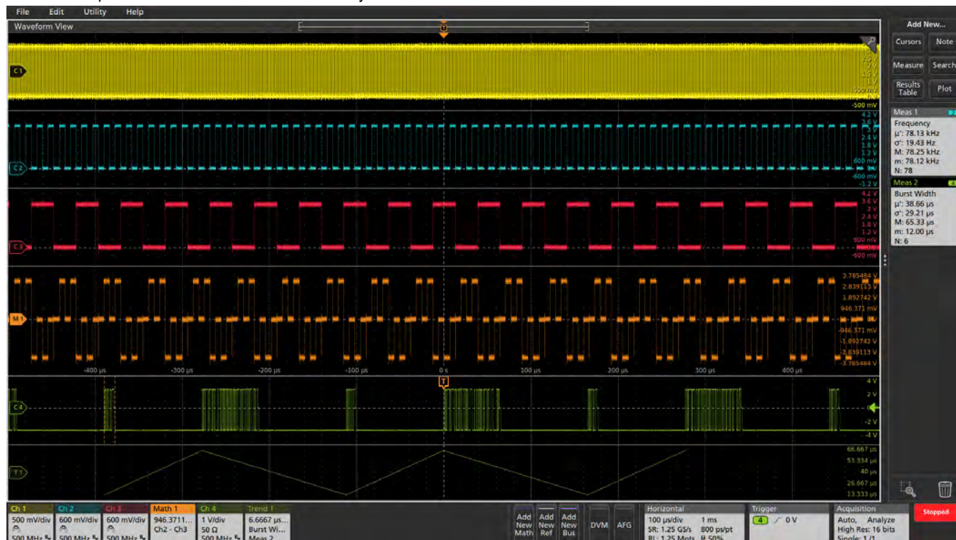
Figure 5: Stacked display mode enables easy visibility of all waveforms while maintaining maximum ADC resolution on each input for the most accurate measurements.
