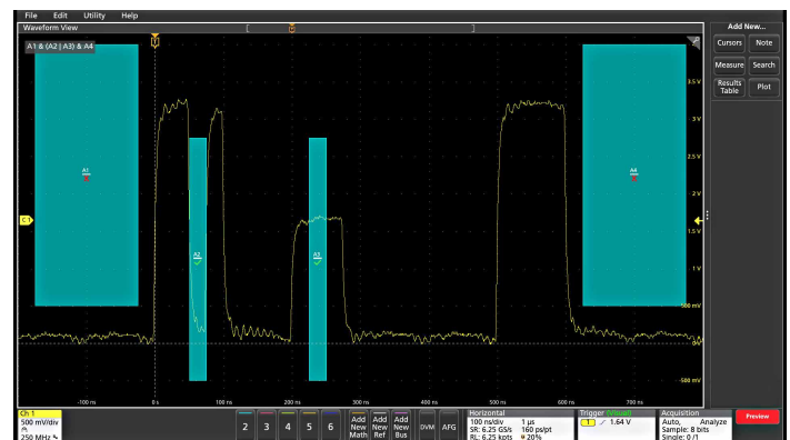
Visual Trigger areas isolate an event of interest, saving time by only capturing the events you want to see.
