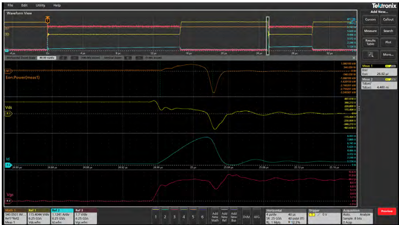
The image shows diode reverse recovery measurements with reverse recovery current and voltage captured on the high-side.
