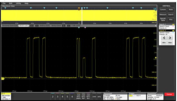
Earlier, FastAcq revealed the presence of a runt pulse in a digital data stream prompting further investigation. In this acquisition, Search 1 reveals that there are six runt pulses in the acquisition.
