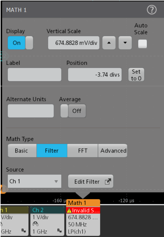
Filters can be created through the Math dialog. Once a filter is edited, it can be easily applied, saved, and recalled for use or modification later.
