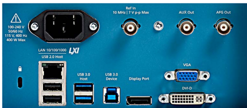
Figure 34: The I/O you need to connect the 6 Series MSO to the rest of your design environment.
