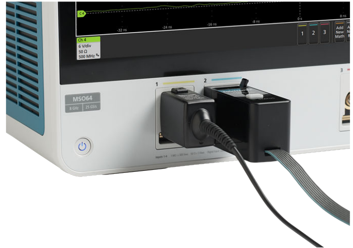
Figure 1: FlexChannel technology enables the ultimate in flexibility. Each input can be configured as a single analog or eight digital channels based on the type of probe you attach.
